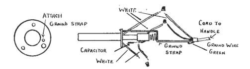
Attach ground strip to heating element. Use small screw and hole nearest barrel. CAUTION: CAPACITOR MUST BE OPPOSITE GROUND STRIP.
