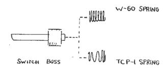
Install spring on Rear Boss of switch. Straight spring Model W-60 conical spring Model TCP-1:
