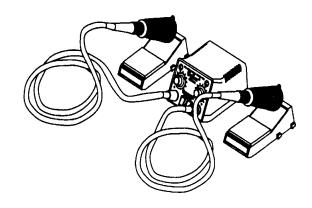
Tip temperature is electronically controlled throughout the temperature range of  $350^{\circ}$ F to  $850^{\circ}$ F ( $175^{\circ}$ C to  $455^{\circ}$ C). The units are calibrated to within  $\pm 10^{\circ}$ F ( $\pm 6^{\circ}$ C) and tip temperature control is maintained within specification over line voltage variations of  $\pm 10^{\circ}$  and an ambient temperature range of  $60^{\circ}$ F to  $110^{\circ}$ F  $16^{\circ}$ C to  $43^{\circ}$ C).
